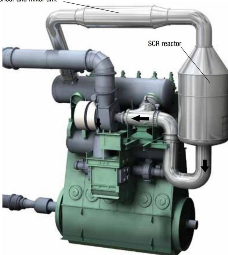
*Illustration of an MAN B&W two-stroke SCR system.*
