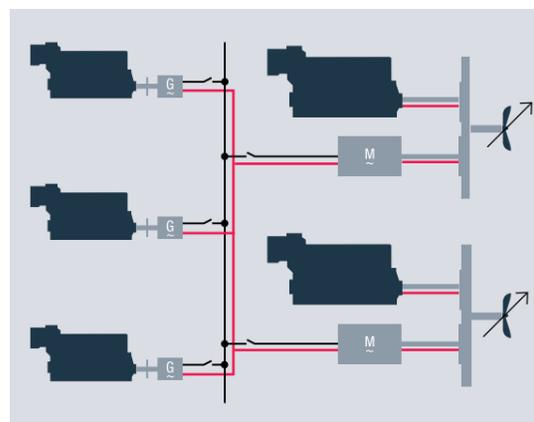
Example: Passenger ferry using a PTI-booster in case of the need for additional power
