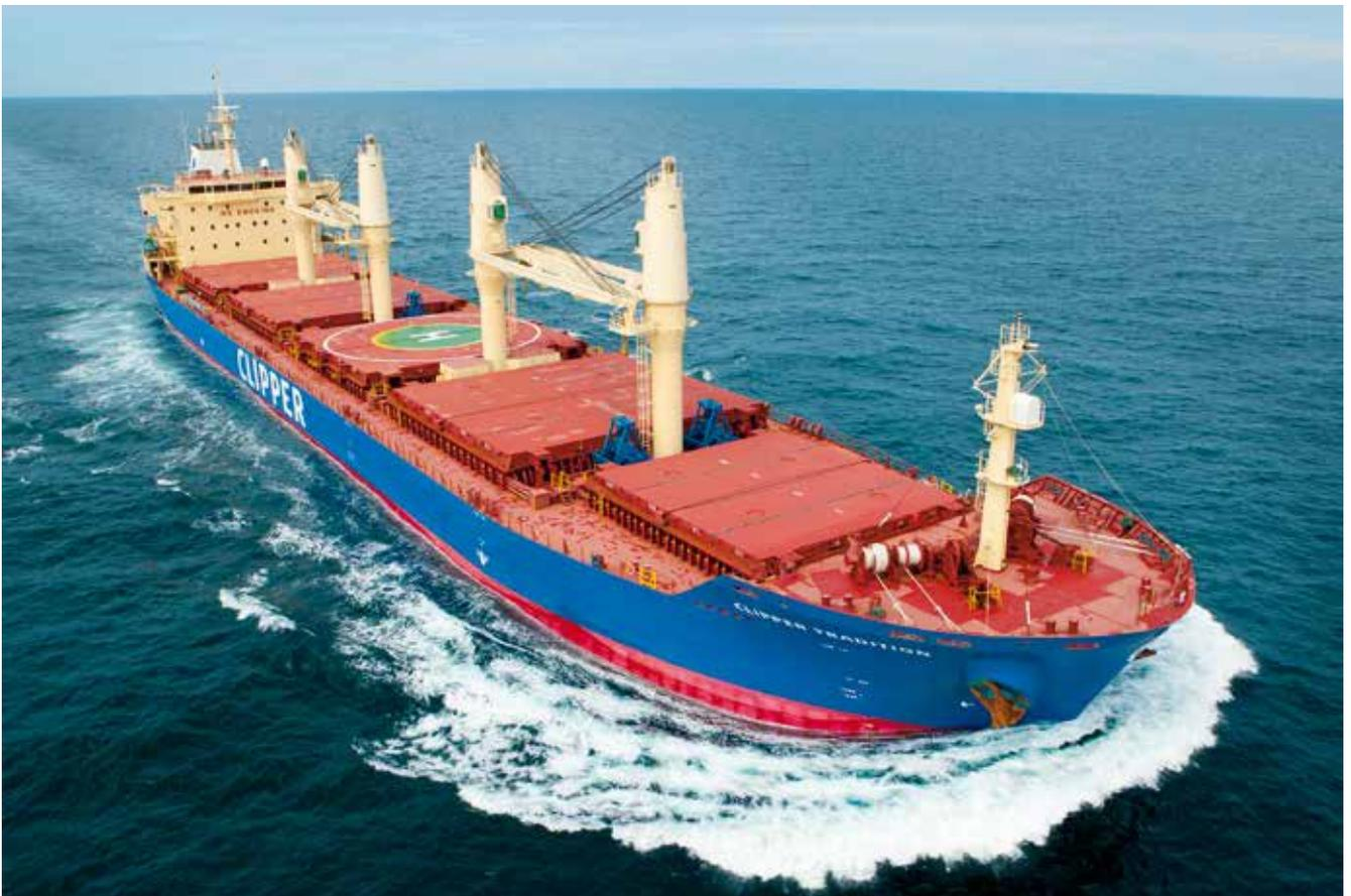
Fig. 1: Handysize bulk carrier
